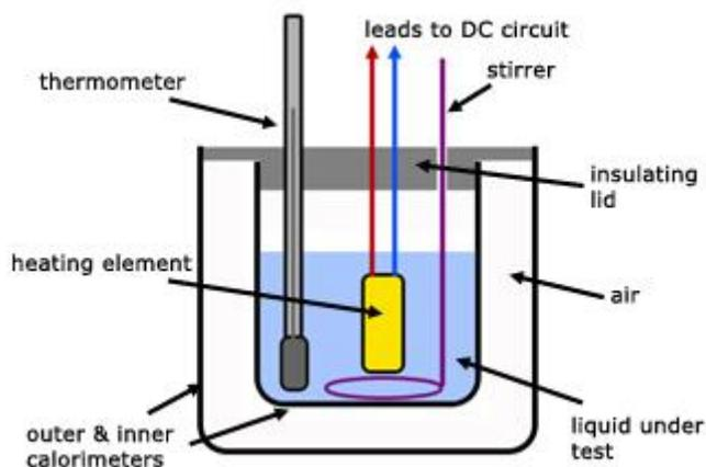
The heat energy supplied by the electrical element is given to the liquid and its container, producing a temperature rise  $\Delta\theta$ .
