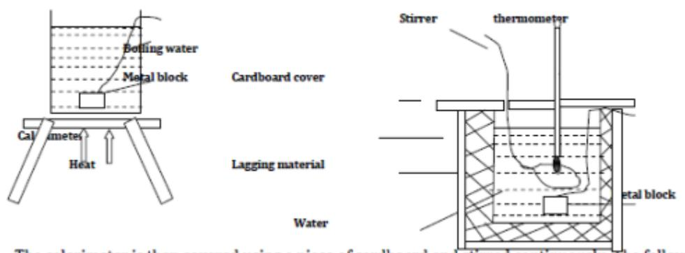
In this method, a known mass of a solid, e.g. a metal block is heated by dipping it in a bath of hot water. After some time, the solid is very fast transferred into cold water in a calorimeter and whose mass is known.
